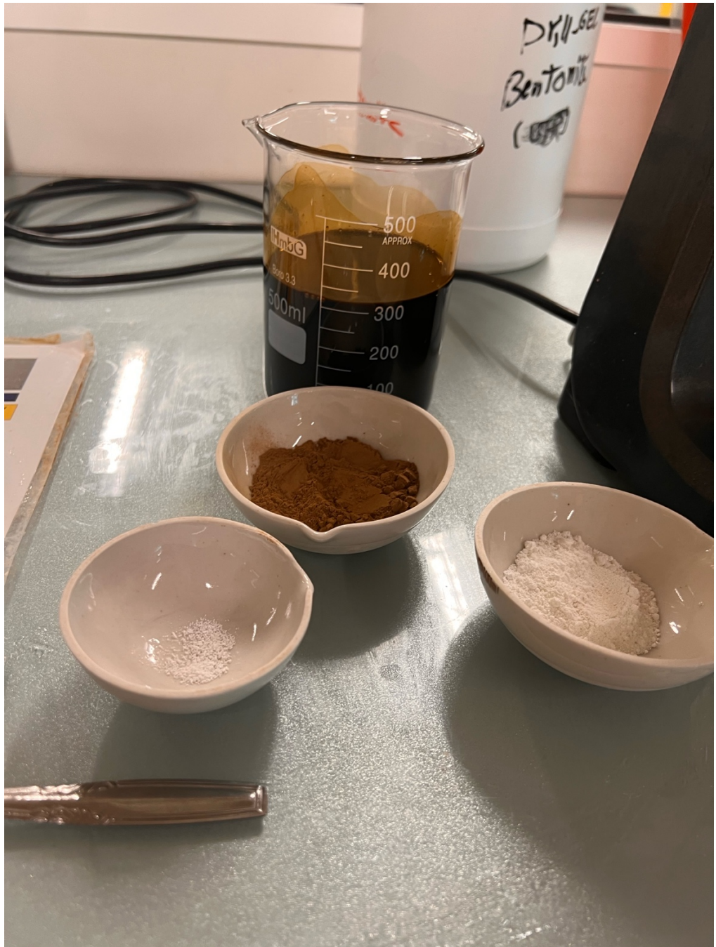
Figure 11: Preparing crude oil base mud
