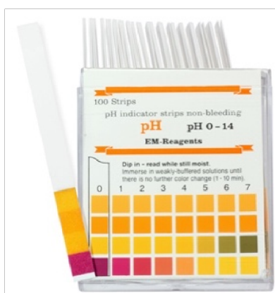
Figure 5: PH PAPER- USING FOR MEASURE PH OF THE MUD.
