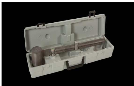
Figure 4: MUD BALANCE FOR MEASURING THE DENSITY
