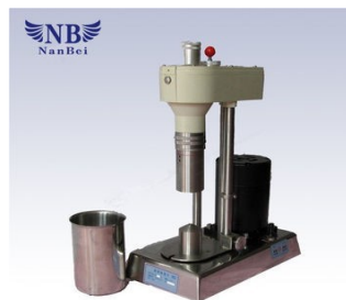
Figure 7: ROTATIONAL VISCOMETER- USED FOR MEASURE THE VISCOSITY OF MUD AT DIFFERENT ROTATIONAL SPEEDS
